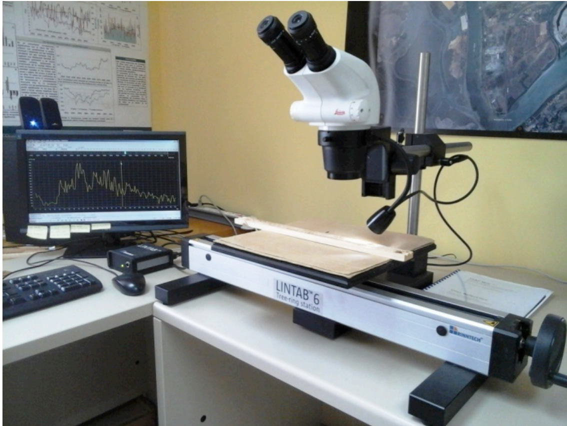
Figure 9. Stereomicroscope and LINTAB™ table, connected to a computer running the program TSAP-Win™.
