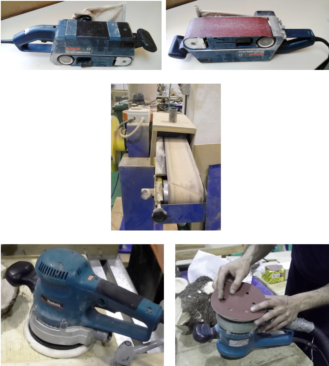
Figure 8. Sanders used to polish the samples. Hand-held sander (top), stationary belt sander (middle), and hand-held random orbital sander (bottom).
