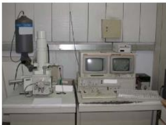
Figure 42. Scanning Electron Microscope JSM-5410
