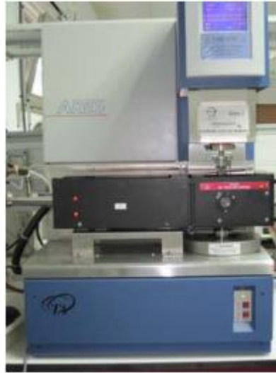
Figure 37. ARES II Controlled Deformation Rheometer
