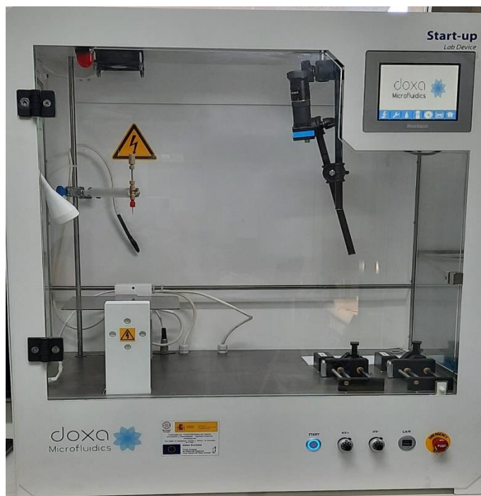
Figure 32. Doxa Microfluidics electrospinning equipment
