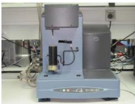
Figure 43. Thermogravimetric balance TGA model Q50
