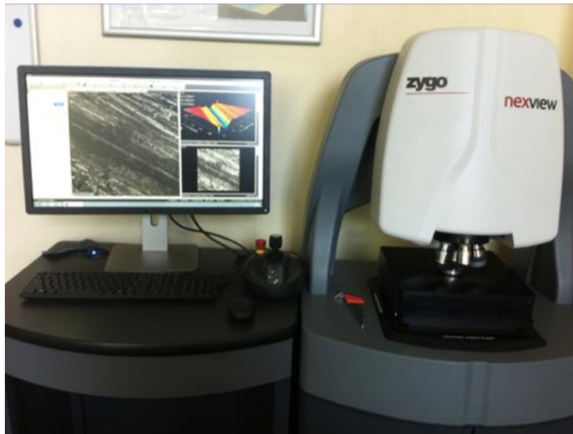
Figure 39. Interferometer Zygo neoview
