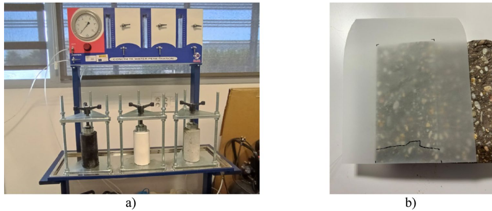
Fig. 1. (a) Water penetration test equipment, (b) Determination of water penetration front of the face.
