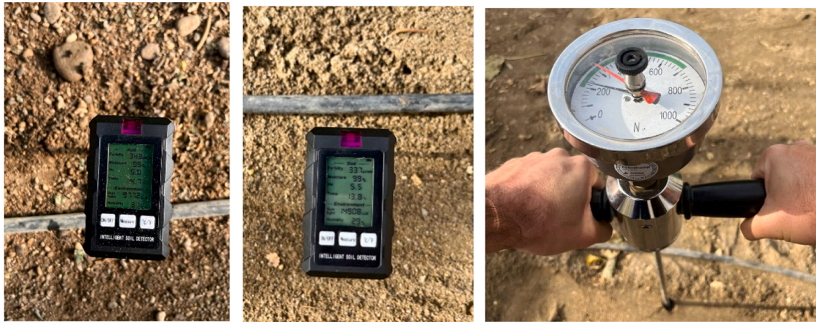
Fig. 6. Soil condition data collection. (a) Sand-covered soil natural of Almeria, (b) Typical sand-covered soil, (c) Durometer.
