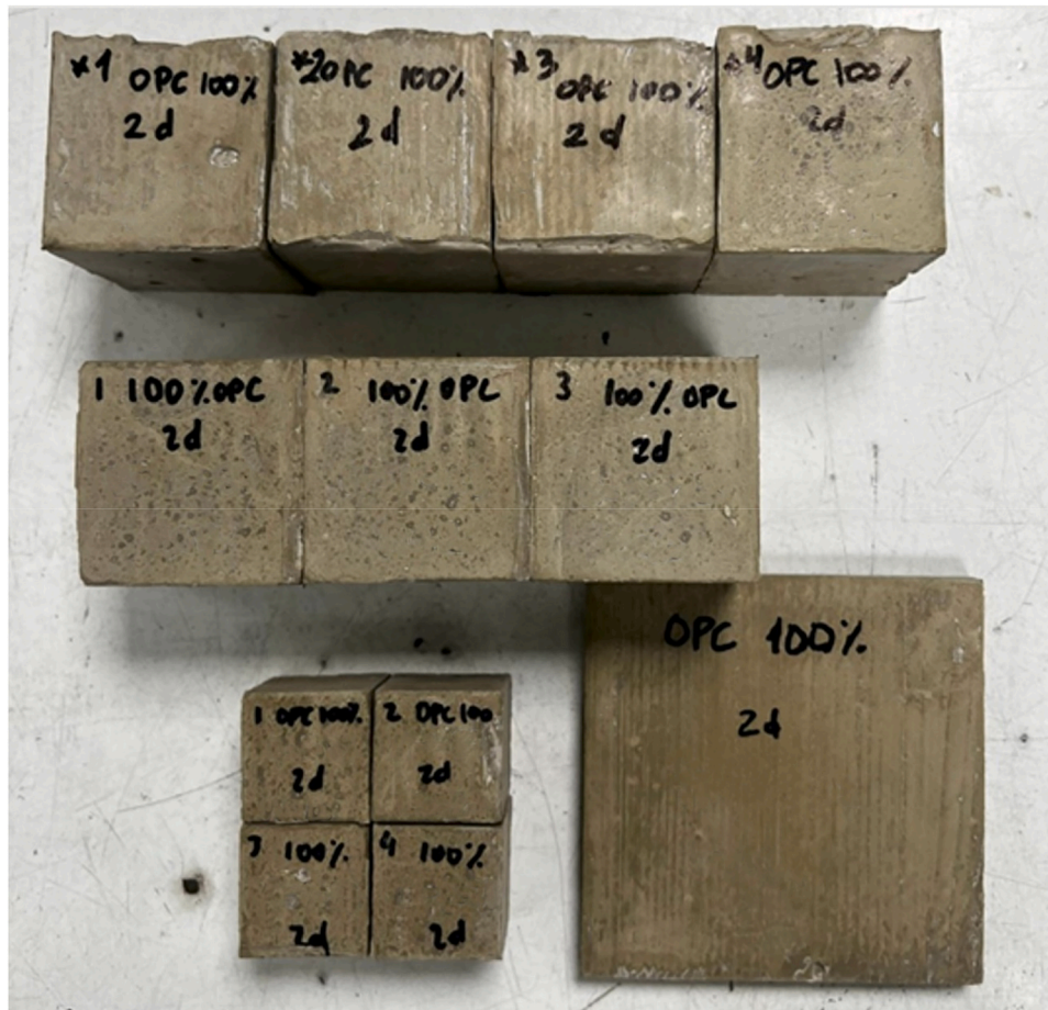
Fig. 3. Example of the samples prepared with the different moulds for the 100-0-2 specimens.
