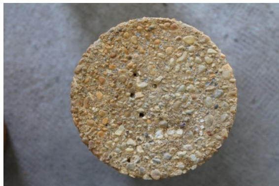
Figure 5. Example of specimens mark (after affecting by AMD).
