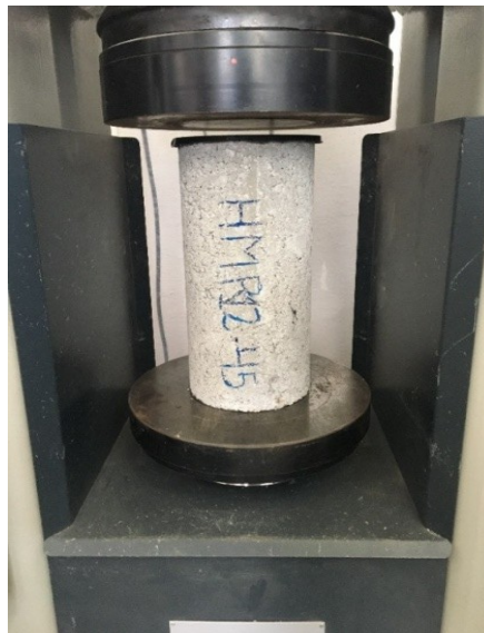
Figure 6. Specimens prepared for the compression test in the press.
