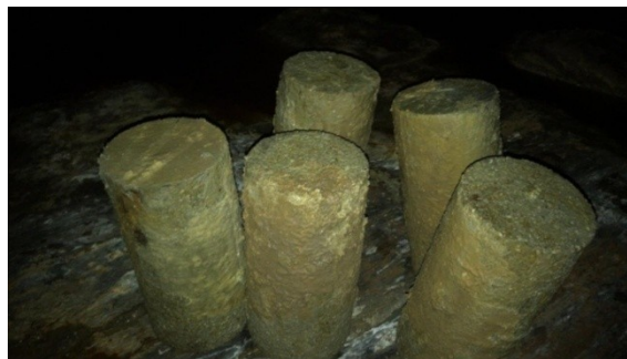
Figure 9. Specimens taken from the water with AMD.
