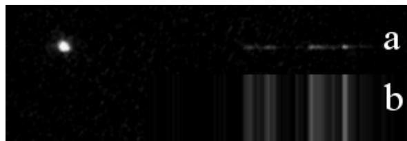
Figure 5. Raw (a) and processed (b) emission spectrum. Order zero appears on the left.
