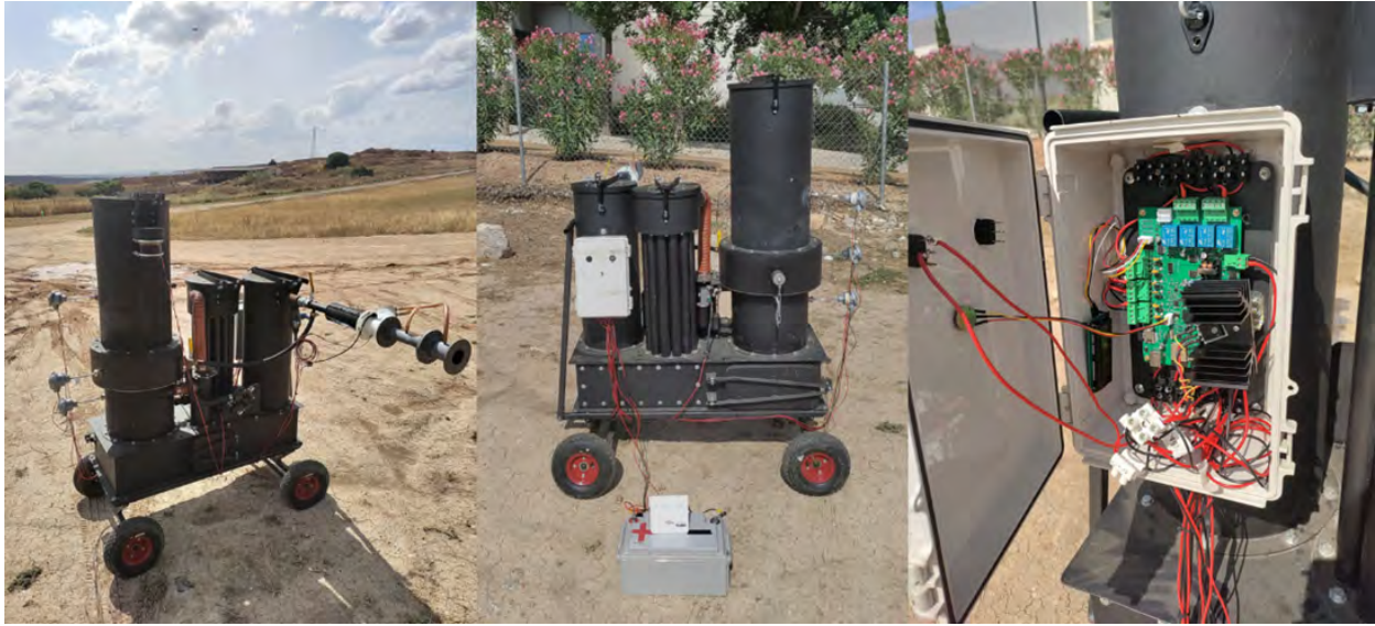
Figure 5: Images of the reactor prototype, including a close-up view of the control system.
