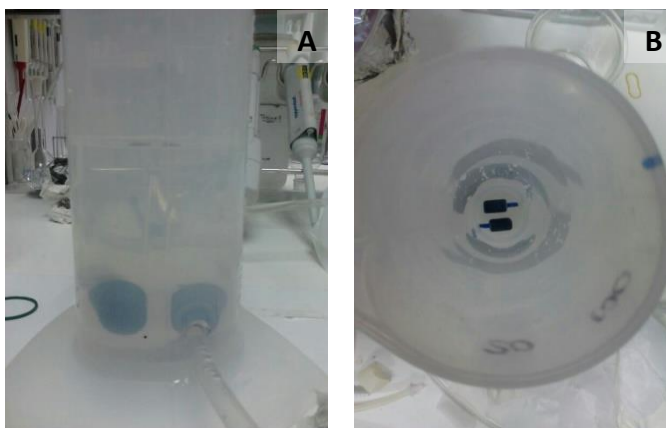
Figure 2.5. (A) Front and (B) top views of the experimental set-up used to perform the foam stability tests. The two small stone-diffusers placed at the bottom of the graduated cylinder are shown.
