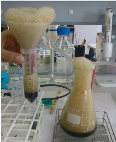
Figure 2.3. Collection in a test tube of the liquid released from the foam after a BSA-added microalgal suspension was bubbled with air during the microalgal partitioning test.
