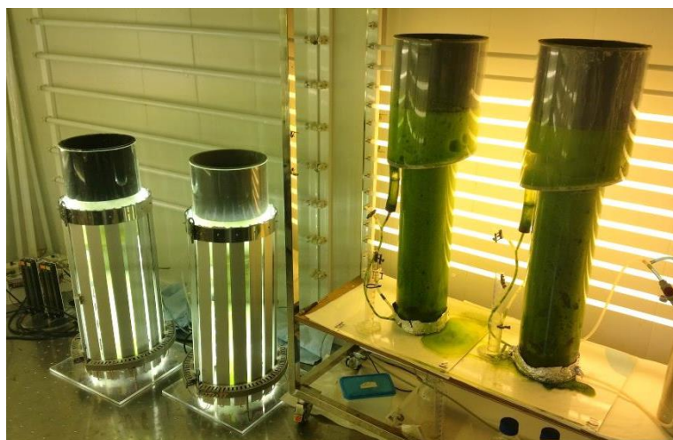
Figure 7.23. Liquid foam-bed photobioreactors illuminated by LED-systems (left, saturating light) and by the fluorescent lamps panel (right, no saturating light).
