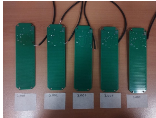
Figure 10. Capacitive soil moisture sensors manufactured by a professional PCB company and coated with AER (green resin in the figure). Designed as 3.001 to 3.005.
