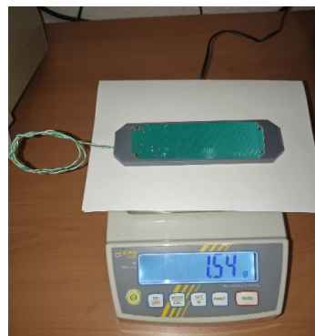
Figure 12. Professionally manufactured sensor with a factory-applied AER layer and an additional manually deposited epoxy coating with a thickness of 0.11 mm (1.54 g of resin).
