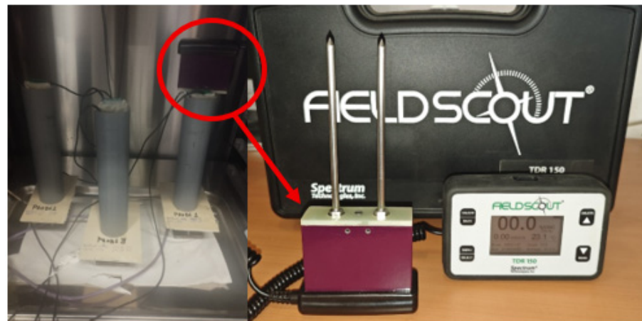
Figure 17. Moisture meter inserted into the test tube to ensure the two calibration endpoints.
