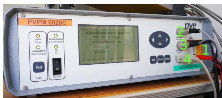
Figure 2. I–V curve tracer, including the PV-Engineering model PVPM-6020C used in the Universidad de Almería. Connection elements: (1) Two four-wire measuring connectors for voltage and current, respectively; (2) input for external Pt100 (module back surface temperature measurement); (3) irradiation input; and (4) RS-232 serial interface to the computer.
