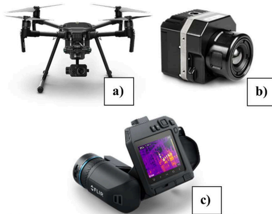
Figure 1.7 – Infrared Thermal Imaging sensors. a) Drone DJI Matrice 300 (SZ DJI Technology Co., Ltd., Shenzhen, China) equipped with FLIR Vue TZ20 b) FLIR Vue Pro for UAV; c) FLIR T865 handheld thermal imaging camera (FLIR Systems Inc., Wilsonville, OR, USA).
