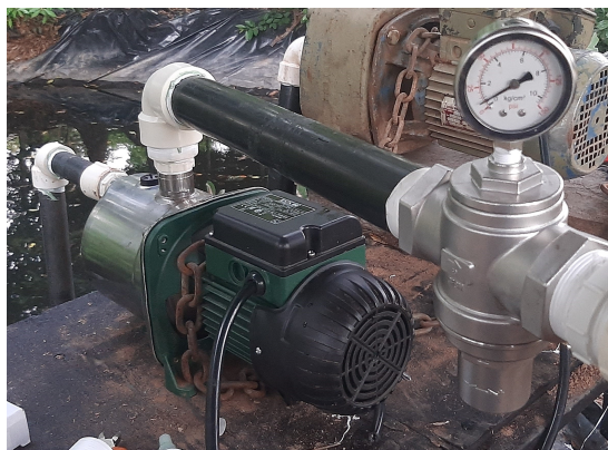
Fig. 4. Photographs of the centrifugal water pump (left) and the electrical cabinet deployed for the experiment
