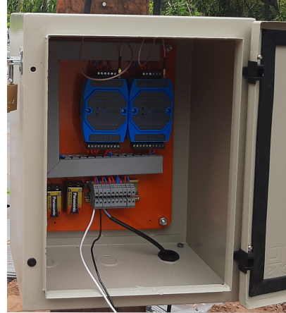
(b) Irrigation node, with two input/output modules employed to control the water pump and to read the flow-meter
