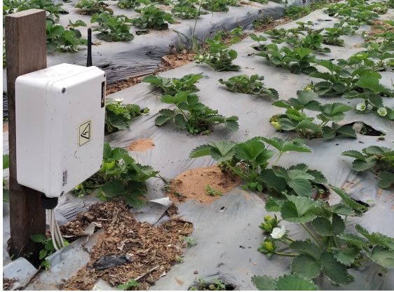
(a) Moisture node. Note the wires corresponding to the soil moisture sensors, that were installed under the ground surface, and the LoRa antenna
