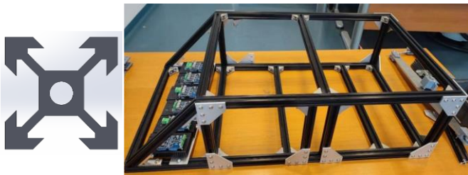
Fig. 2. a) Section of modular aluminium profile. b) Manufacture of the central chassis of the terrestrial robotic platform.
