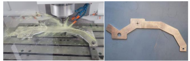
Fig. 3. Machining Process on CNC Centre of Moving Part for Robotic Platform
