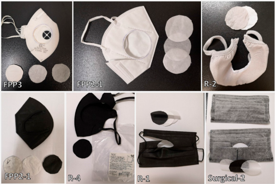
Figure A2. Example of facemaks and their respective circular sections and layers.
