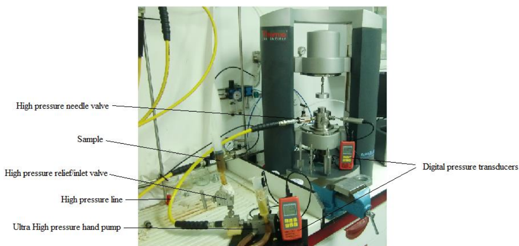
Figure 3. 6. Picture of the pressurization system 1 connected to the pressure cell mounted in the MARS II rheometer
