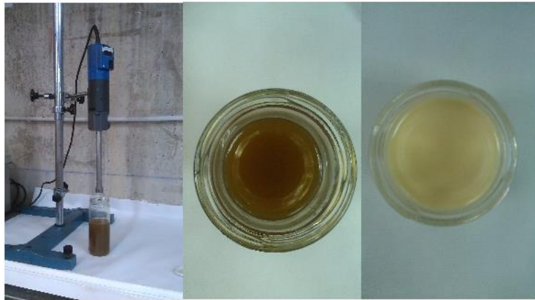
Figure 3. 2. High-shear processing set-up sketch; All-oil suspension picture and Invert-mud picture
