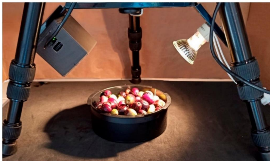
Figure 2. Example of an olive sample measurement taken during the spectral data acquisition.
