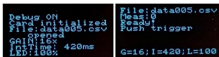
Figure 2. Image of the device's integrated OLED screen showing initialization data (left) and ready to perform data capture (right).
