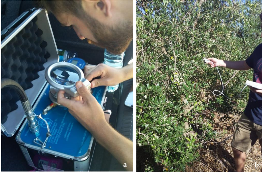
Figure 4. Images of reference parameters measurement process; a) \Psi_{PD} with the pressure chamber, b) g_s with the leaf porometer.
