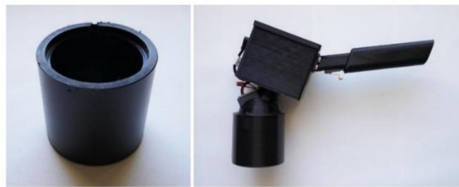
Figure 3. Images of the measuring container alone (left), and fitted with the device's dome during measurement (right)
