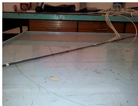
Figure 7. Sealing testing with sensors immersed in water.
