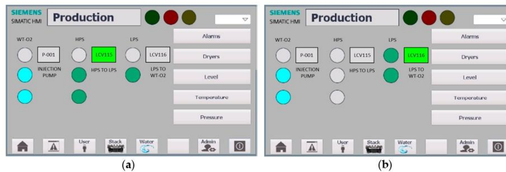
Figure 14. Hydrogen production subsystem monitoring interface: (a) mid-level in HPS, valve (LCV115) open; (b) high level in LPS, valve (LCV116) open.
