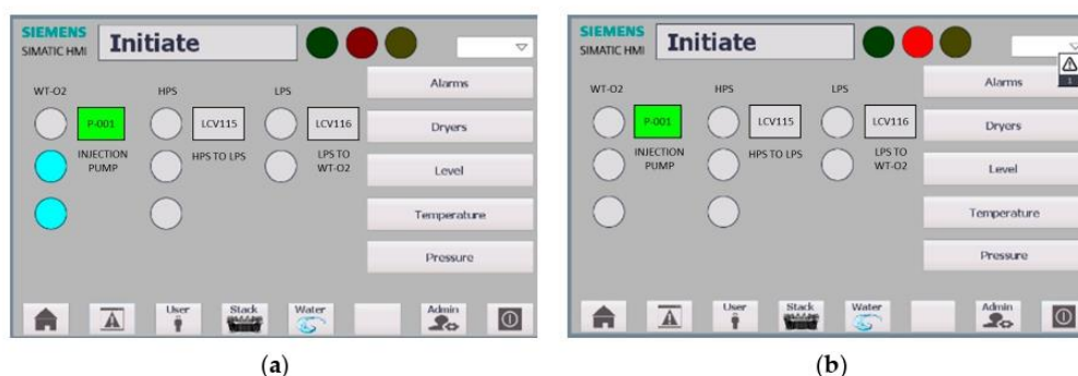
Figure 12. Water management subsystem monitoring interface: (a) normal operation; (b) low level alarm.
