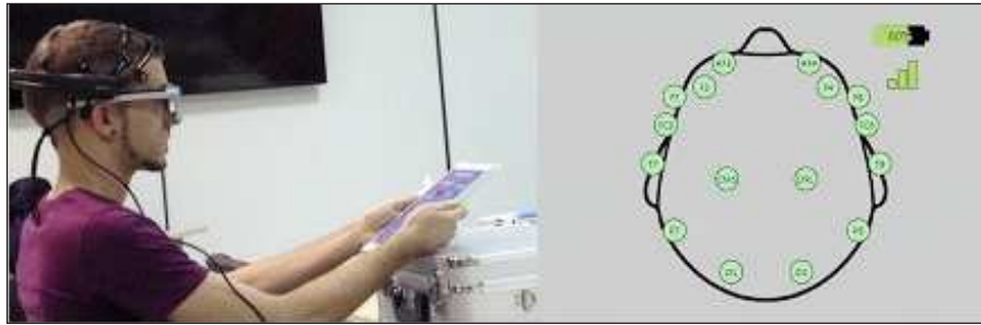
Figure 2. Simultaneous monitoring of the EEG and "Eye Tracking", and the position of the EEG sensors.
