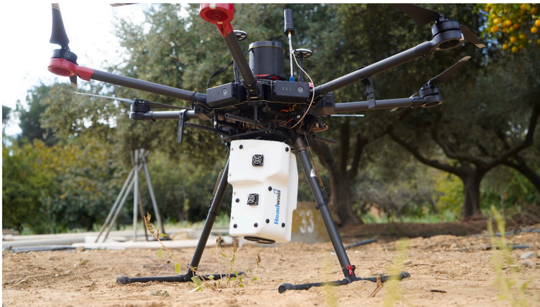
Fig. 1. DJI Matrice 600 Pro UAV equipped with Headwall Hyperspec Co-Aligned VNIR-SWIR hyperspectral camera.
