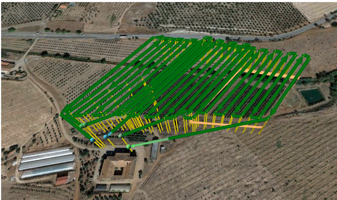
Fig. 2. 3D illustration of the flight mission plan over the experimental olive grove, as planned in the UgCS software interface. The green lines indicate the drone's flight path.
