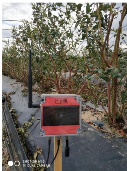
Figure 7. Installed device taking measurements every 30 min.
