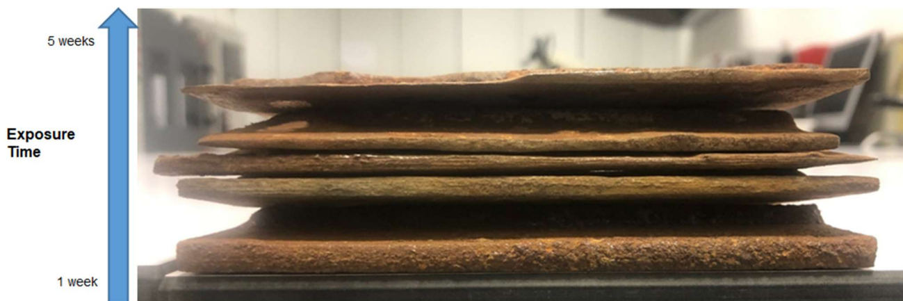
Figure 3. Evolution of volume loss in test specimens submerged in the same AMD river.
