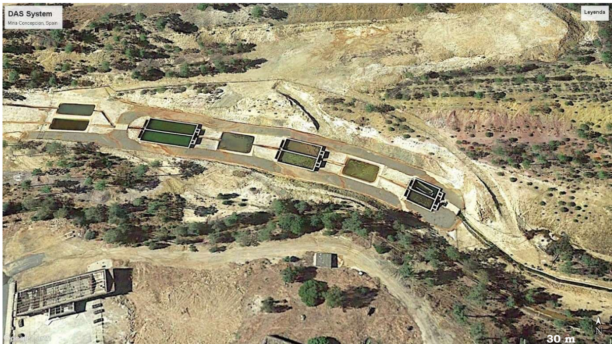
Figure 3.2 Aerial image of a passive water treatment plant using dispersed alkaline substrate (DAS) technology to remediate acid mine drainage in Huelva, Spain (Google Earth Pro, 2020).
