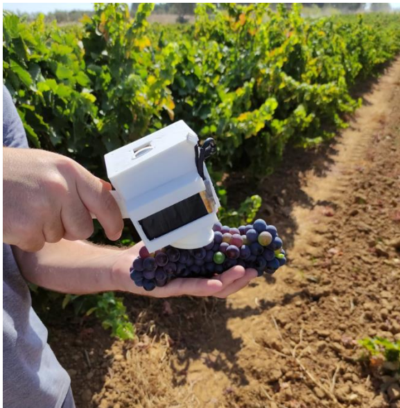
Fig. 2. Proposed multispectral device during data acquisition
