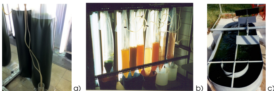
Figure 3.2. Polyethylene bags used for Diacronema vlkianum growth (a) and Chlorella vulgaris carotenogenesis (b); Outdoor raceway ponds for Chlorella growth (c).
