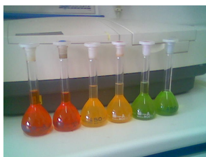
Figure 3.6. Haematococcus pluvialis and Chlorella vulgaris (orange and green) acetone extracts used for total pigment spectrophotometric determination.
