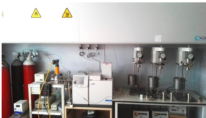
Figure 4. Supercritical fluid plant (left) with the gas chromatograph and the three high pressure reactors (right).
