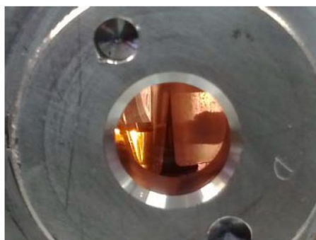
Figure E7. Inside the reactor: catalyst (right) and EDA (left) location, fixed to the stir axis.
