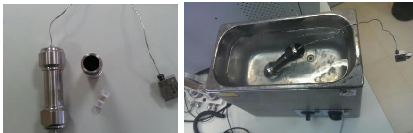
Figure 14. Left: HPLC column system. Right: Sonication bath with HPLC column inside.
