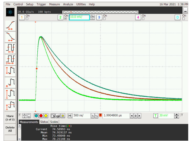
FIGURE 11. Transient response of the CSA for an input charge of 30 fC. Tunability of the decay time.
