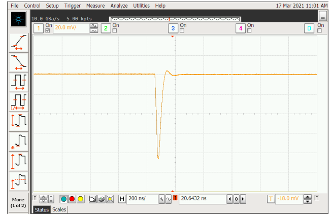
FIGURE 14. Measured response at the fast shaper output.
