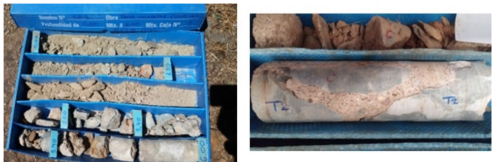
Fig. 13 Sounding witness box and detail of them, of the Calabazar Dam
