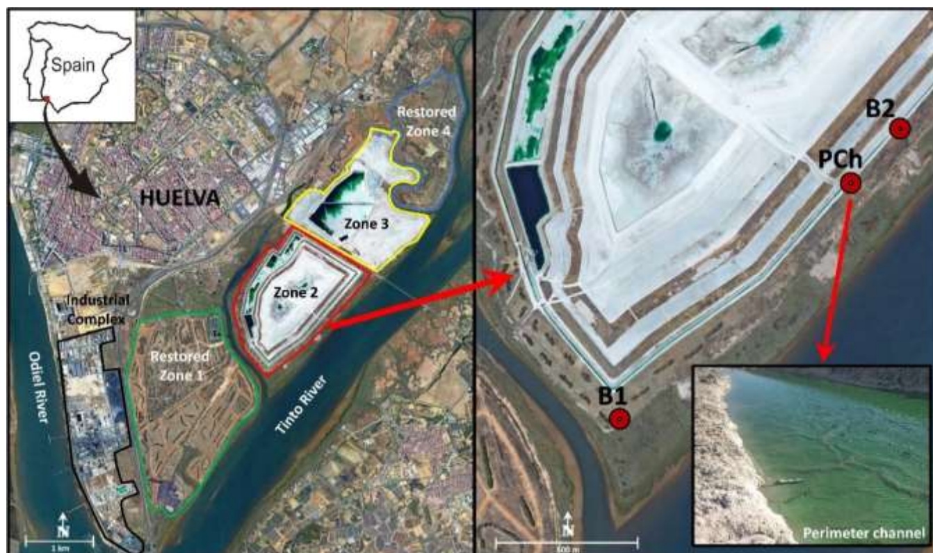
Figure 1. Location map of the Huelva phosphogypsum stacks and location of the phosphogypsum leachates sampling points: Boreholes (B1 and B2) and perimeter channel (PCh) located in the zone 2 of the phosphogypsum stacks of Huelva.
