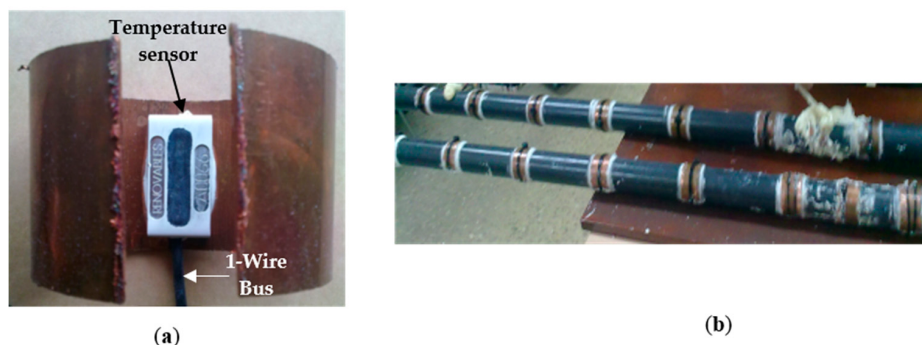
Figure 5. (a) Temperature sensor attached to the metal ring; (b) GTP disassembled into two sections and arrangement of the sensors on the probe.
