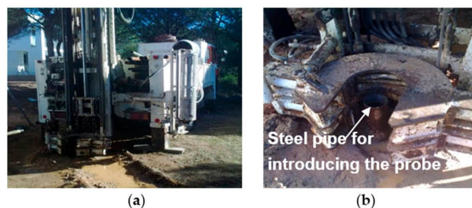
Figure 9. (a) Drilling machine; (b) Steel pipe for introducing the probe.
