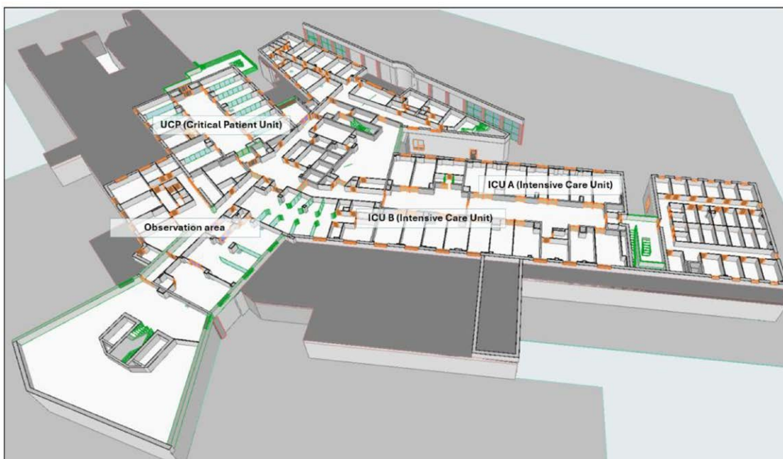
Figure 2. BIM model of the workspace in Archicad 28. BIM = building information modeling, CPU = critical patient unit, ICU = intensive care unit.
