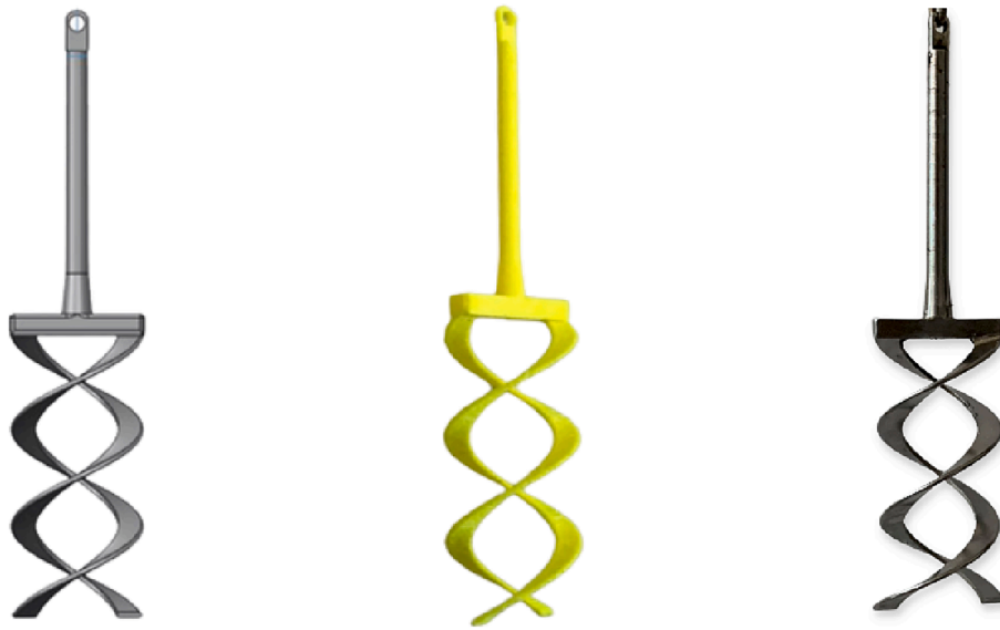
Fig. 3.7. DHR solid model (left), 3D printed prototype (centre) and stainless steel (right).
