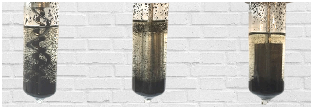
Fig. 1.1. Rheological measurement problems with practical oil-particles emulsions using different testing geometry, a dual helical impeller on the left, a cylindrical spindle in the centre (SC-27) and a vane spindle on the right. Initially, the sample contained in the tubes may be homogeneous. After some time, the sample may become quite stratified.
