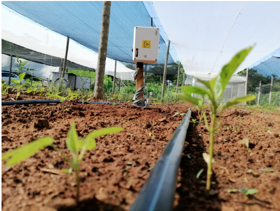
(a) Pure sensing node with moisture sensors
