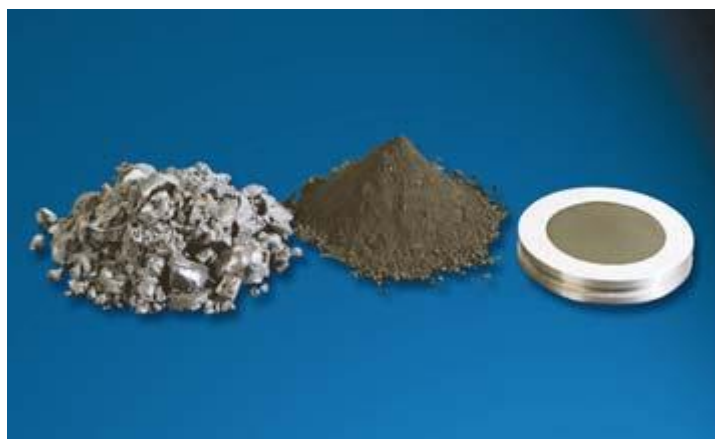
Figure 2.4. Sample preparation for XRF analysis.
