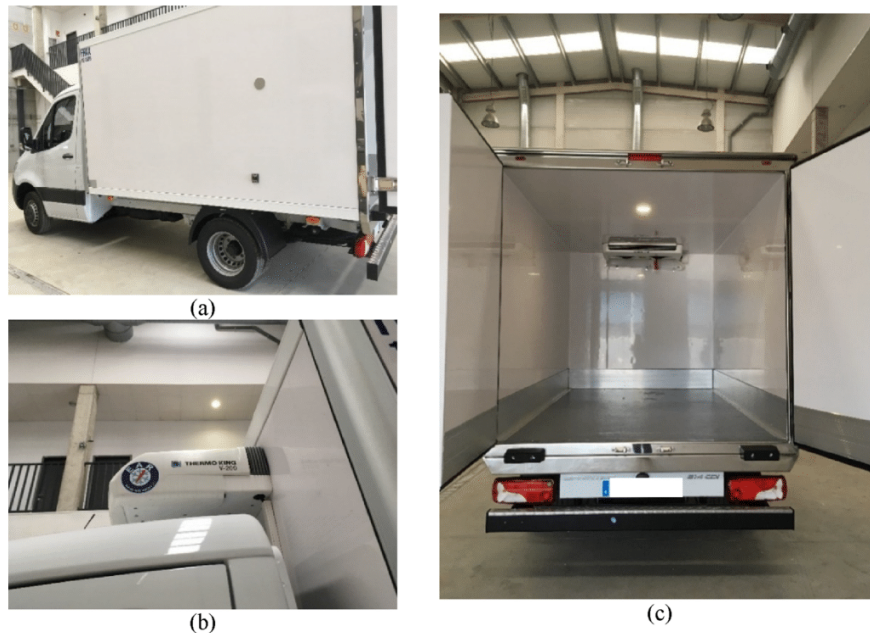
Fig. 11. (a) Detail of the light refrigerated truck; (b) electric refrigeration system; (c) isothermal cool box.
