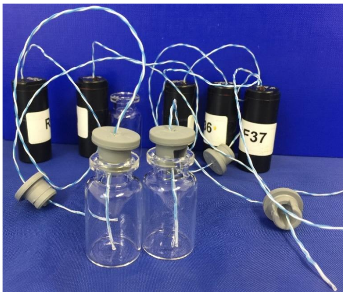
Figure 17. Wireless thermologgers used for product temperature measurements throughout the studies.
