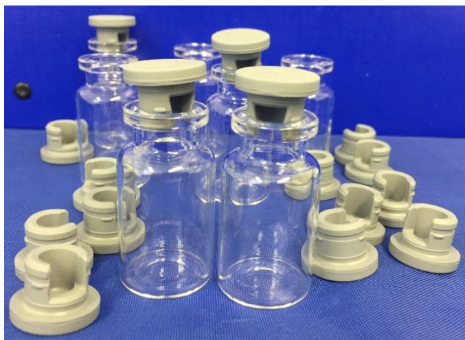
Figure 15. Container-closure system (10-mL vials and igloo single vented stoppers) used in all freeze-drying experiments.
