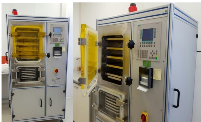
Figure 16. HOF laboratory freeze dryer used throughout the studies.
