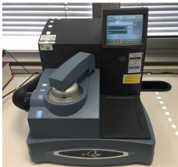
Figure 18. Q2000 series differential scanning calorimetry used throughout the studies.
