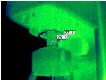
Figure 3.10: Thermal image of rheometer MCR 302 during operation [141]
