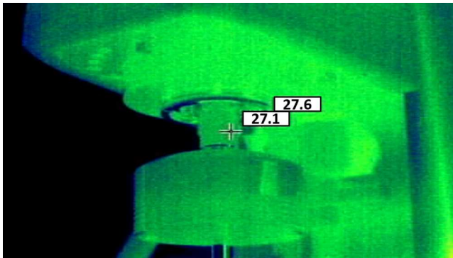
Fig. S1 Thermal image of rheometer MCR 302 during operation.
