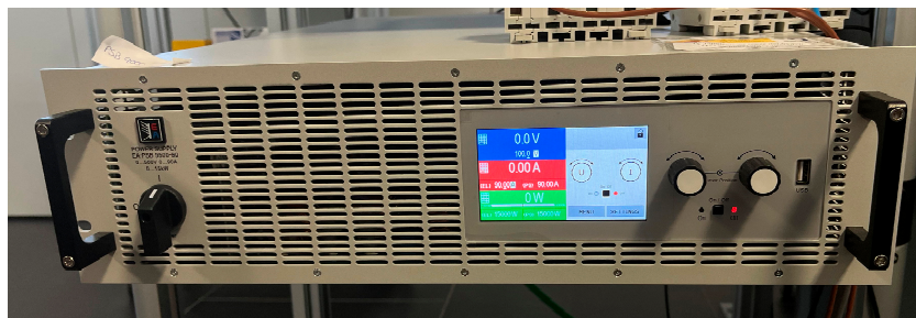
Figure 9. Bidirectional power supply that emulates a Li-ion Battery.
