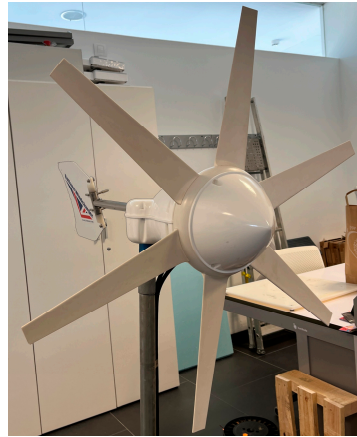
Figure 6. Wind turbine model (Rutland FM910-4) used in the experimental setup.
