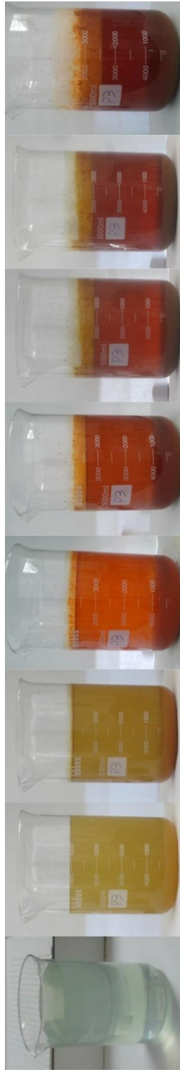
Figure A.1.4: AMD evolution between all Fe in solution as Fe(II) (left) to Fe(III) (right). The ochre color in the first steps indicate that the solution is over saturate in schwertmannite and the red color in final steps show that the solution is equilibrate with Fe(III).
