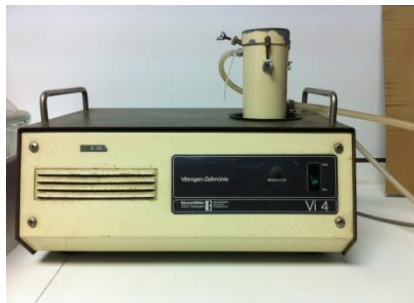
Figure 18- Bühler homogenizer used in the preparation of crude extracts from cultures of C.onubensis .
