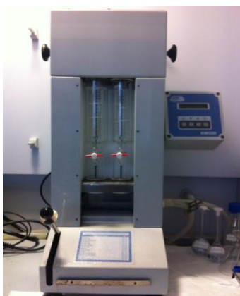
Figure 14. Multi-point grease extractor or automatic soxhlet.
