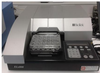
Figure 12. Well-plate reader used to measure optical density of the different B. braunii cultures at 680 nm and 750 nm.
