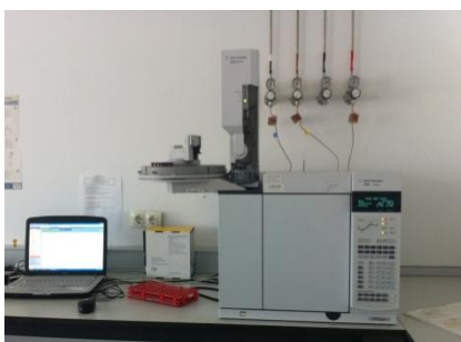
Figure 16. Gas chromatography equipment used for hydrocarbons quantification.
