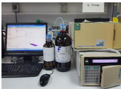
Figure 13. High-performance liquid chromatography equipment (HPLC) used for the separation and quantification of specific carotenoids.
