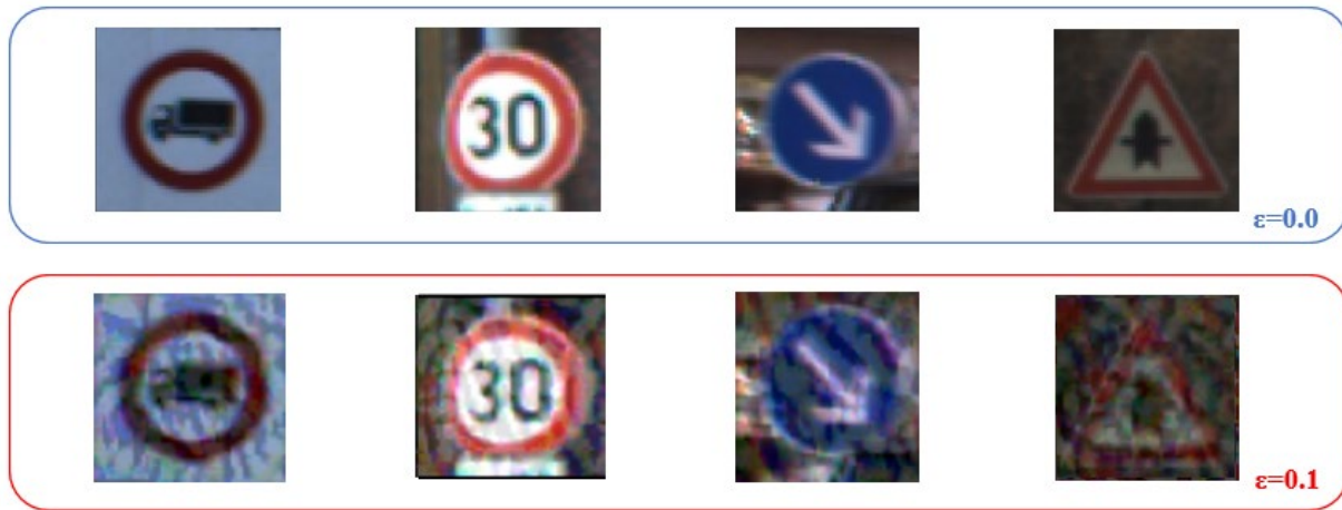
Figure 4. PGD adversarial attacks on the traffic sign classification task for different \epsilon values.
