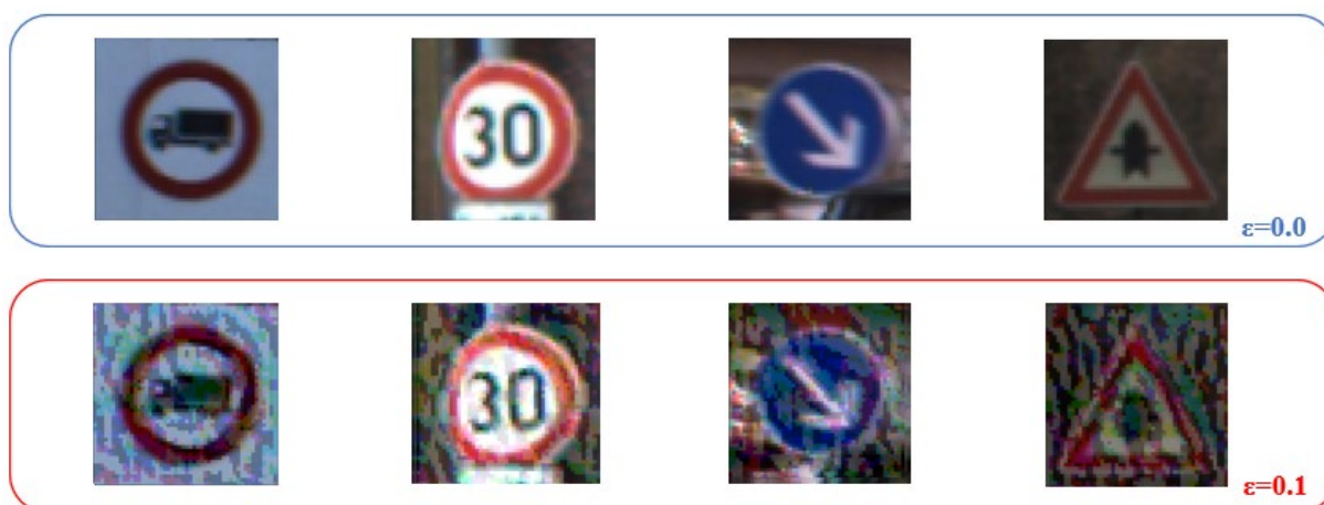
Figure 3. FGSM adversarial attacks on the traffic sign classification task for different \epsilon values.
