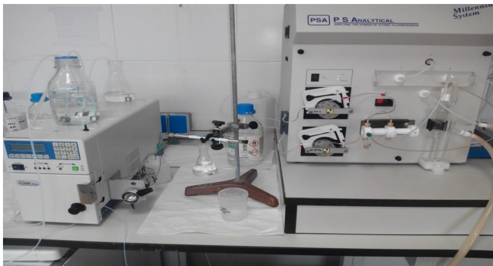
Fig. 3.6. Instrumental coupling of HPLC-HG-AFS which is used in the present thesis.
