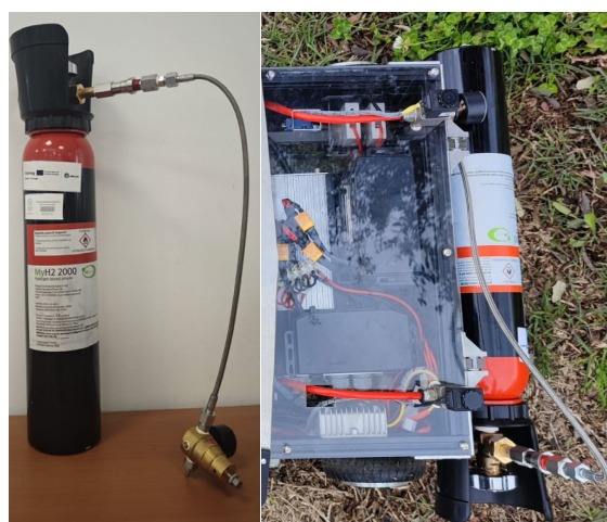
Figure 9. Detail of the hydrogen tank MyH2-2000: (left) in the laboratory; (right) outdoors, on the Hygrobot platform.
