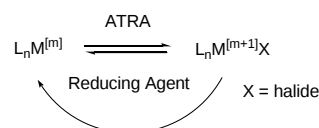
Scheme 5. Catalyst regeneration in metal-mediated ATRA reactions.
