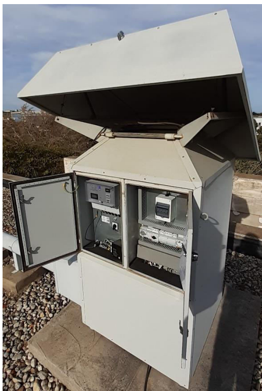
Figure 2.3.2.1. Very high-volume air aerosol sampler, model ASS-500 (on the left), and tray used to place filter SQ inside the air sampler (on the right).
