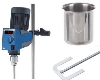
Figure 42. Controlled-rotational speed mixing device, anchor impeller and open vessel used in the processing of oleogels
