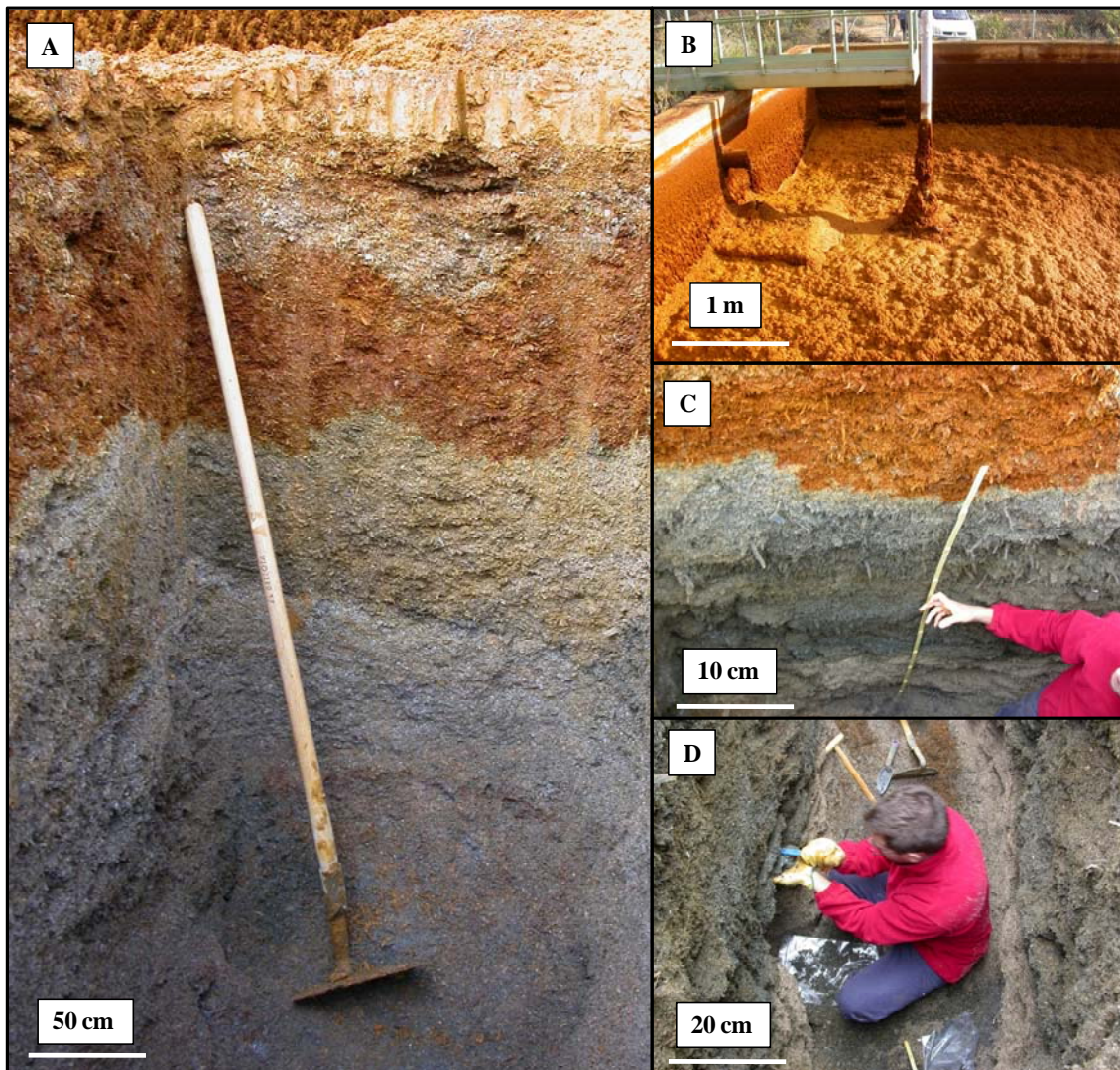
Figure A3.8. A) Reactive tank cross section. B) Iron precipitates on the reactive material surface. C) Reactive material profile characterization. D) Sampling of the different precipitates observed within the reactive material.
