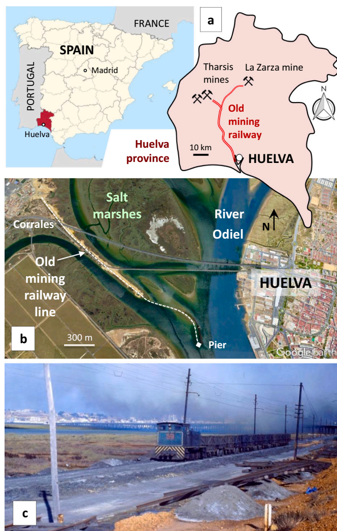
Fig. 1. Locality map showing the old railway line of the Tharsis mines (a). The study area is located on the western bank of the salt marshes of the Odiel River (b), along the last section of the former railway corridor (c), where an uncontrolled quantity of pyrite ore was stockpiled on the ground and spilled from the mining rail cars (photo ca. 1970, Aljaraque Municipality Archive).
