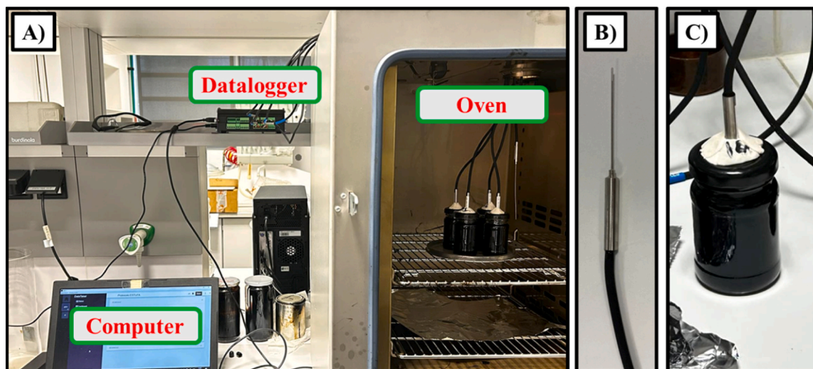
Fig. 1. A) Set-up for the indoor thermoregulation tests, B) Pt-100 temperature sensor, and C) sample jar with an embedded Pt-100 sensor.
